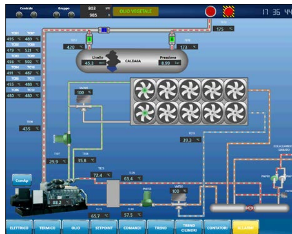
Movicon.NEXt oversees heating and fuel filtration, heat recovery from engine cooling water and exhaust fumes.
